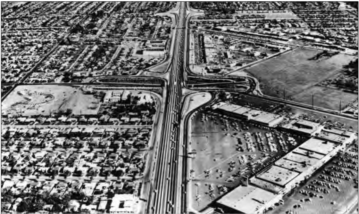
Figure 12. Development densely concentrated along the San Bernardino Freeway. The original West Covina Center was oriented along Garvey Ave. with a shallow setback (background). The later portion of West Covina Center (foreground) was set back from Garvey Ave. in a V shape with surface parking on each side. Aerial photograph was taken in 1960, looking east (Source: Los Angeles Public Library)
