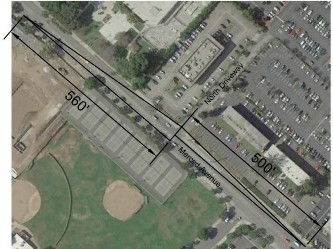
Figure 8. Sight Visibility Triangles
